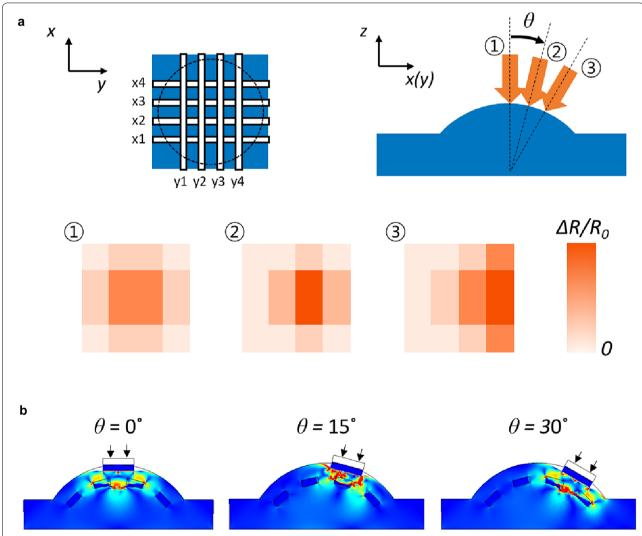
**Fig. 2** Working principle of the proposed sensor. **a** Multi-layer liquid metal microchannels in x (x1, x2, x3, and x4) and y (y1, y2, y3, and y4) direction and different loading directions in x(y)-z plane. Different responses of the sensor array with respect to the loading direction (①, ②, and ③). **b** Finite element analysis (FEA) simulation results showing the corresponding deformations of the liquid metal microchannels
