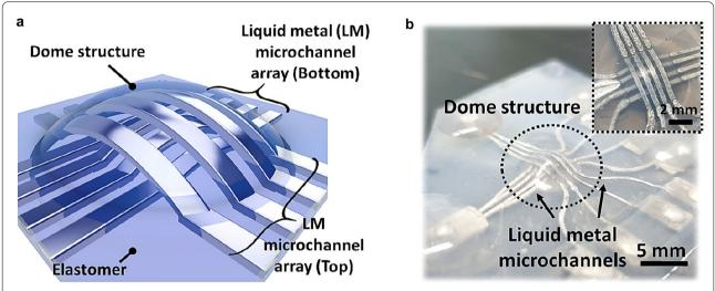
Fig. 1 Liquid metal-based multiaxial force sensor with dome structure. a Schematic design of the proposed sensor. b Images of the proposed sensor
