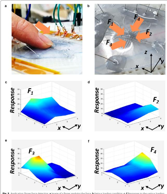
Fig. 5 Application: finger force detection. a Image of a finger applying the force. b Various loading condition. c-f Responses to the various loading forces
