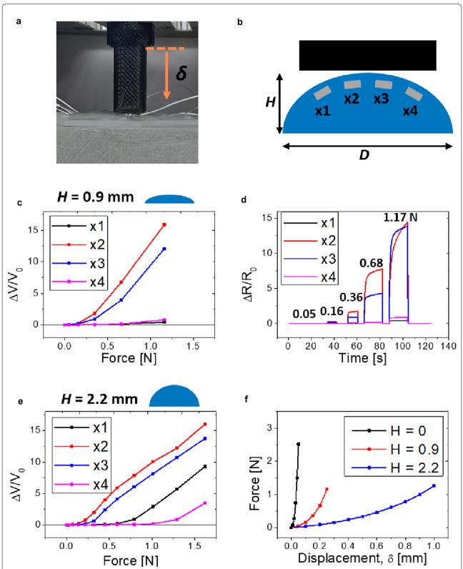
**Fig. 4** Performance characterization. **a** Experimental setup. **b** Schematic view of the sensor. (x1–x4: labels for each LM microchannel, *H*: height of the dome, and *D*: diameter of the dome) **c** Response of the sensor with the dome height (*H*) of 0.9 mm to normal directional force. **d** Real-time response to various loadings **e** Response of the sensor when *H* is 2.2 mm. **f** Sensitivity to the displacement according to the height of the dome
