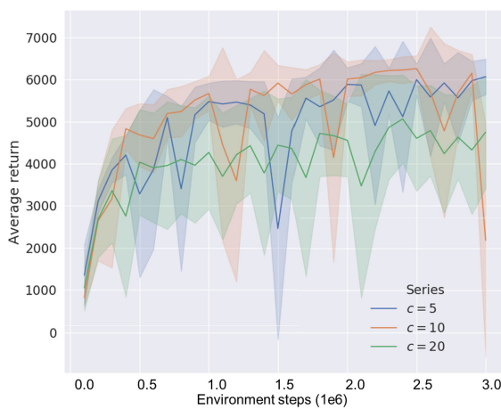
FIGURE 11. Learning curves for Ant-v2 environment using SAC-FER algorithm with different c = D_{KL,max} values.
