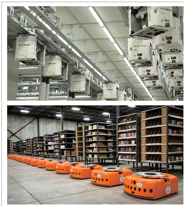
[ Figure 1 ] Semiconductor factory logistics transport robot (top), automatic warehouse warehouse logistics transport robot (bottom)
