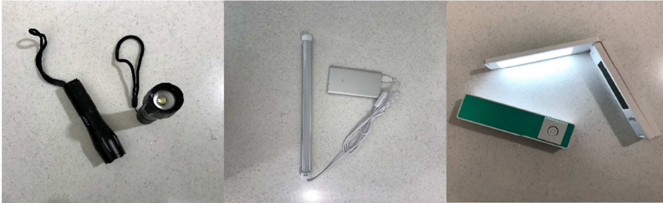
Figure 4. Lighting variations: (Left) point lighting, (center) line lighting, (right) plane lighting
