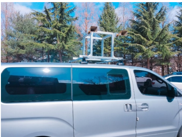
Fig. 5. The picture of the SAR measurement setup in an automobile.
