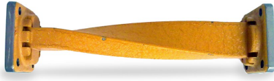
Figure 6: Twisted waveguide section (90 degree). A structure consisting of several straight sections connected by 180 degree twists is predicted to have a high geometric factor close to C \approx 0.6 in a dipole magnet while avoiding many engineering challenges of other setups.
