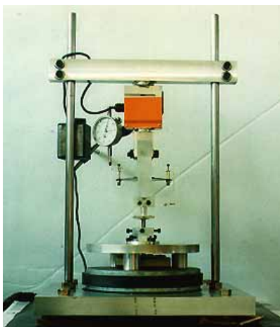
Figure 16. Electromagnetic actuator and the load frame of the vibration-fatigue testing system
