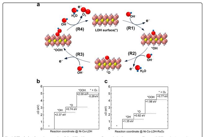
Fig. 2 DFT calculated reaction energies of the OER with corresponding optimized structures. a The overall OER mechanism on the surface of LDH in alkaline media and reaction energy diagram of the OER. Energy profiles of each reaction step on **b** the Ni–Co-LDH monolayer slab and **c** Ni–Co-LDH–RuO<sub>2</sub> nanohybrid
