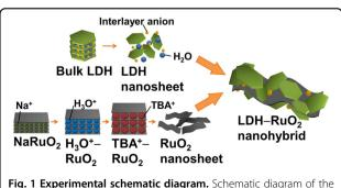
**Fig. 1 Experimental schematic diagram.** Schematic diagram of the exfoliation-restacking route to LDH–RuO<sub>2</sub> nanohybrids
