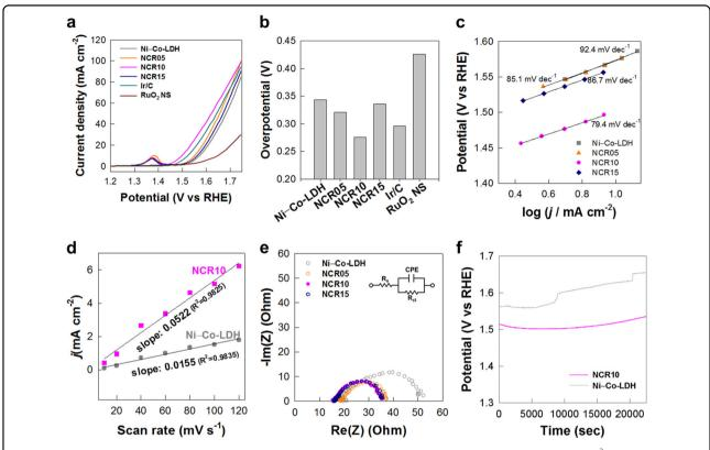
Fig. 5 Electrocatalytic properties of the NCR nanohybrids. a LSV curves. b Overpotential required to reach  $j = 10 \text{ mA cm}^{-2}$ . c Tafel plots of NCR nanohybrids and Ni–Co-LDH. d Charging current density differences plotted against scan rates of NCR10 and Ni–Co-LDH. e EIS spectra of NCR nanohybrids, and f chronopotentiometry measurements at  $j = 10 \text{ mA cm}^{-2}$  of NCR10 and Ni–Co-LDH
