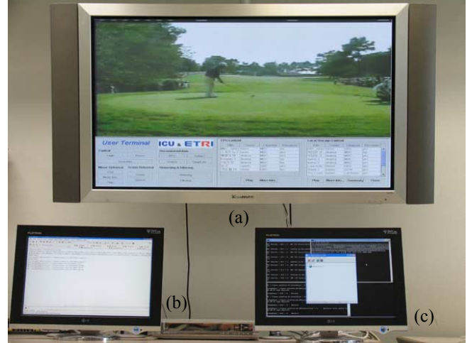
Fig. 4. An intelligent broadcasting system applied with agent platforms: (a) User Terminal, (b) Service Information Provider, and (c) Service Provider.
