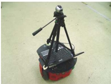
Fig. 7 Experimental platform – Pioneer II robot with a single camera.
