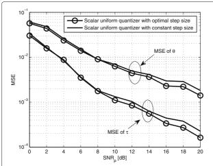
**Fig. 6** MSE of joint phase and timing estimation versus  $SNR_p$  in the presence of scalar fronthaul quantization and joint phase and timing estimation (31): F = 2, C = 3, A = 0.7, N = 100 and  $N_p = 16$
