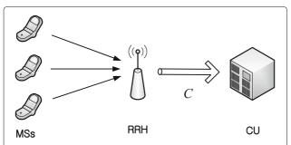
**Fig. 1** Uplink communication between a number of MSs and an RRH. The RRH is connected via a finite-capacity fronthaul link to a CU that performs baseband processing, including synchronization
