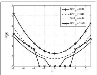
**Fig. 2** Inverse of the PSD of the quantization noise obtained from Algorithm 1 versus the frequency index k: C = 3 bits/sample, F = 2, A = 0.7, N = 100 and  $N_D = 16$
