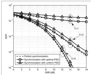
**Fig. 4** SER with uncoded BPSK transmission versus SNR with joint phase and timing estimation (31): F = 2, A = 0.7, N = 100 and  $N_p = 16$
