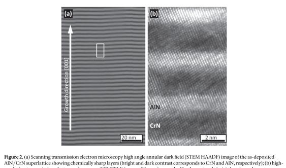
AlN/CrN superlattice showing chemically sharp layers (bright and dark contrast corresponds to CrN and AlN, respectively); (b) h resolution transmission electron microscopy (HR-TEM) image of the region marked by the rectangle in (a) showing coherent multilayers. The multilayers are stacked along the [001] direction.
