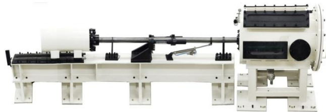
Figure 5 Single stage gas gun developed
