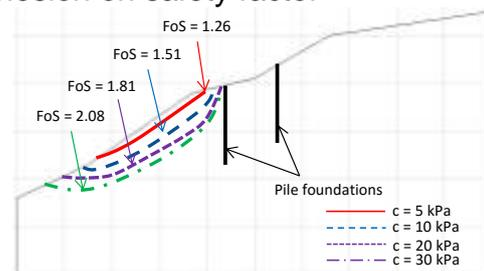
Figure 11. The slope failure mechanisms after 70 hours of rainfall (1.08 cm/h)
