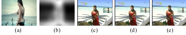
Figure 7. Effect of the informative blending. (a) the frame to be inserted, (b) saliency map of (a), (c) no blending, (d) prob. blending, (e) informative prob. blending.
