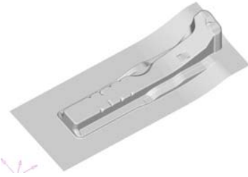
Figure 2. CAD model of the tool for the stamping of the member (initial binder design).
