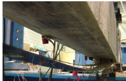
(b) Full debonding of the CFRP layer following load step 14
