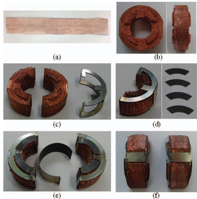
FIG. 3. Manufacture process of half-split-type radial-thrust combo MMFB. (a) Copper metal mesh. (b) Top and side views of compressed combo metal mesh damper. (c) Half-split combo metal mesh damper and stainless steel plates. (d) Combo metal mesh damper covered by stainless steel plates and thrust top foils. (e) Combo metal mesh damper with welded thrust top foils and radial top foil. (f) Side view of combo MMFB.
