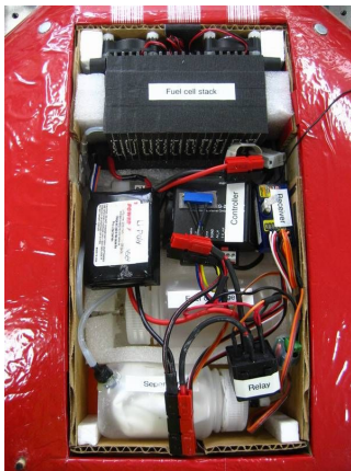
Fig. 5. Integration of the fuel cell system into a UAV test bed.
