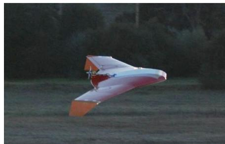
Fig. 7 Blended Wing Body-type UAV Test bed
