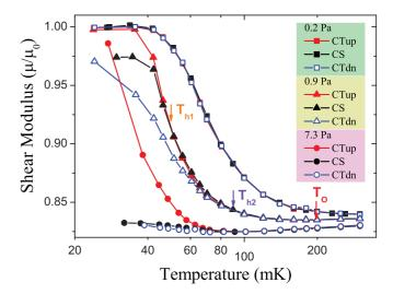
FIG. 2. (Color online) Shear modulus with various thermal and mechanical trajectories as a function of temperature. Color codes represent different protocols (thermodynamic histories).
