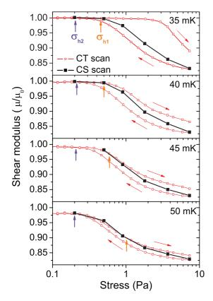
FIG. 3. (Color online) Shear modulus in solid <sup>4</sup>He at various temperatures. Red squares are values under decreasing stress (CTdn) and subsequent increasing stress (CTup). Black squares were obtained during CS scan.
