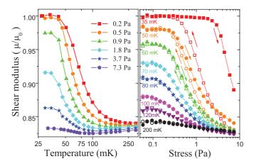
FIG. 1. (Color online) (a) Shear modulus measured under constant stress scans at various stress values. (b) Shear modulus measured by sweeping stress values down and up at various temperatures.
