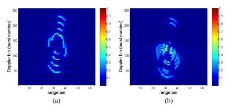
Figure 6. Conventional FT-based ISAR imaging of ideal point-scatterers: (a) set 1 and (b) set 2.
