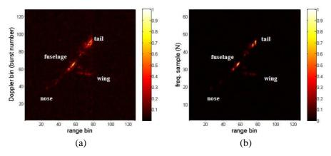
Figure 11. Application results of the measured B-727 data using: (a) FT and (b) DGR with Q = 32.
