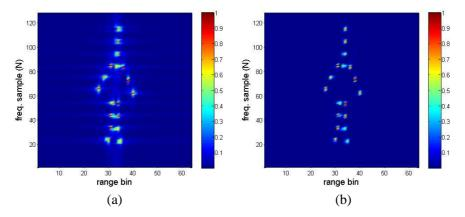
Figure 7. ISAR images of the ideal point-scatterer set 1 using: (a) STFT and (b) DGR with Q = 32.
