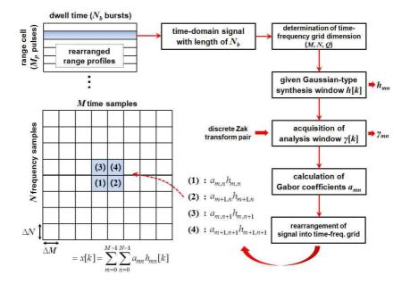
Figure 3. Diagram for application of the oversampled DGR to the rearranged 2D radar received signal.
