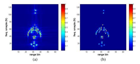
Figure 9. ISAR images of the ideal point-scatterer set 2 using: (a) STFT and (b) DGR with Q = 32.
