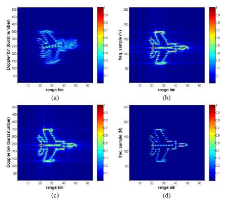
**Figure 10.** Simulation results of the MIG-25 using: (a) FT, (b) STFT, (c) GWT and (d) DGR with Q = 64.
