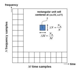
**Figure 2.** DGR time-frequency grid with a size of  $(N \times M)$  and sampling intervals with respect to  $N_b$ .
