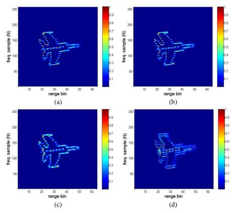
Figure 12. Simulation results of the MIG-25 at a different temporal frame using the DGR when Q is given as: (a) 128, (b) 64, (c) 32 and (d) 16.
