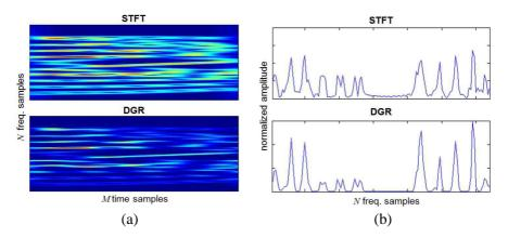
Figure 8. Comparison between the STFT and the DGR using the time-domain signal at the selected 35th range cell: (a) time-frequency plots and (b) Doppler profiles.
