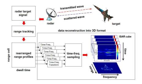
Figure 1. Overall procedures of the TFT-based ISAR imaging.
