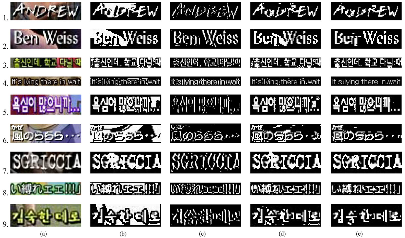
Fig. 19. Results of overlay text extraction (a) Original image. (b) Otsu result. (c) Sato filtering result. (d) Lyu result without the height normalization. (e) Our approach.
