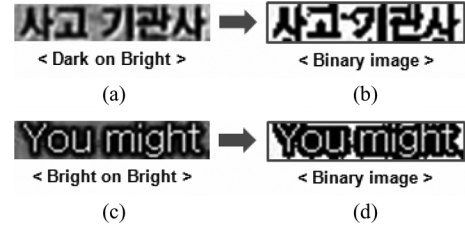
Fig. 11. Examples of binarized image by the average intensity of overlay text region.
