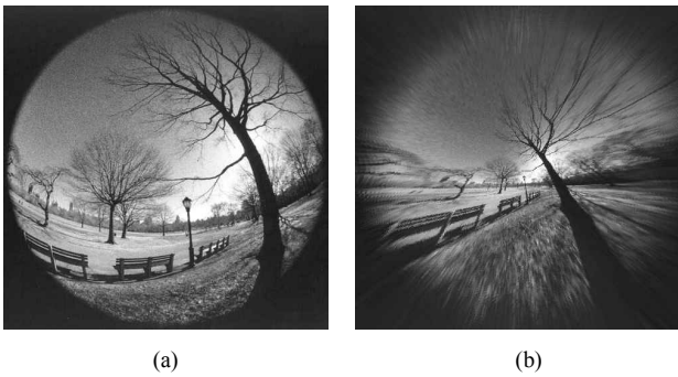
Figure 6. Correction result of a circular wide-angle image (size: 486 \times 486 ). (a) Distorted image from Fig. 1-(a). (b) Undistorted image corrected by the improved FOV model.
