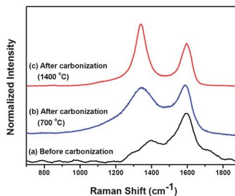
Fig. 3 The Raman spectrum of CNT/carbon nanofibers (a) after being electro-spun and air-stabilized at 250 °C, (b) heat-treated at 700 °C and (c) 1400 °C for carbonization.
