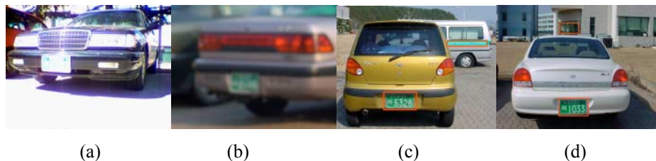
Fig. 8. Examples of LP detection with mistakes: LPs were missed due to bad illumination (a) and excessive blurring (b). False detections are present in (c) and (d) where white characters were written on green background and complex color patterns occurred in glass, respectively
