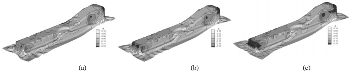
FIGURE 4. Distribution of the thickness strain on the inner panel with the variation of the blank holding force: (a) BHF = 100 kN; (b) BHF = 200 kN; (c) BHF = 300 kN.
