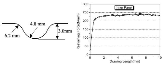
**FIGURE 8.** The restraining force of the draw-bead in the inner panel
