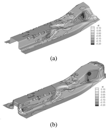
**FIGURE 6.** Distribution of the thickness strain with respect to the initial blank: (a) open channel type; (b) semi-open channel type;
