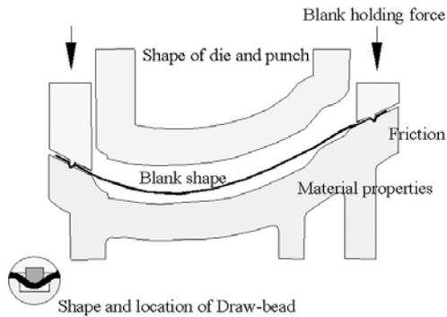
**FIGURE 1.** Process parameters in the sheet metal forming
