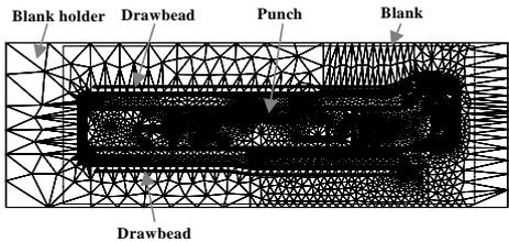
**FIGURE 9.** Locations of draw-bead in the sheet metal forming die for an inner panel.
