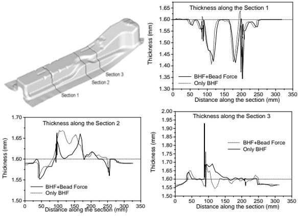
**FIGURE 11.** Comparison of thickness distribution with respect to the presence of draw-bead.
