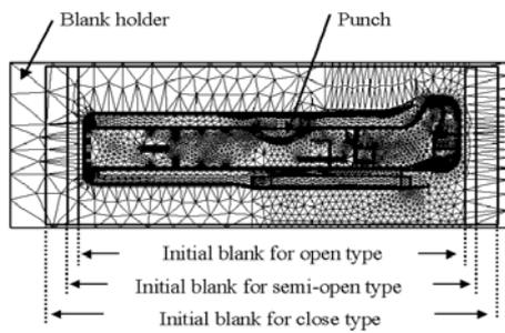
**FIGURE 5.** Initial blank for the forming analysis of an inner panel with open and semi-open type.
