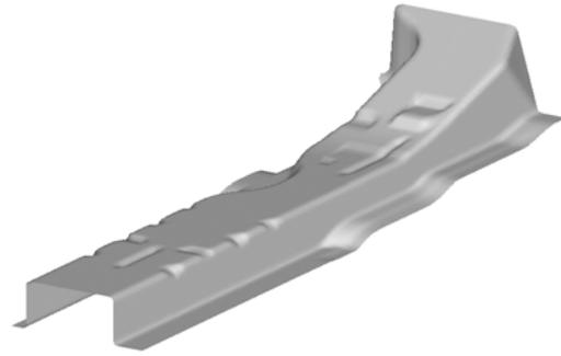
**FIGURE 2.** Shape of the inner panel in front frame member
