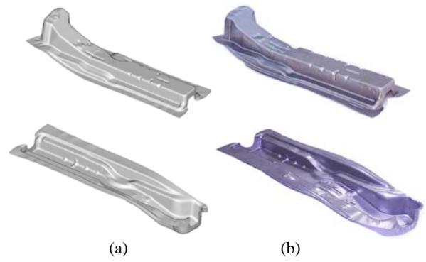
**FIGURE 12.** Comparison of the deformed shape for the experimental verification: (a) analysis result; (b) real product
