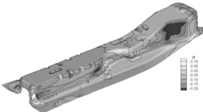
**FIGURE 10.** Thickness strain distribution of the inner panel when the draw-bead force is applied
