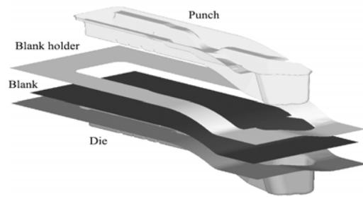
FIGURE 3. Initial setting of tools and the blank for the numerical analysis of the inner panel.
