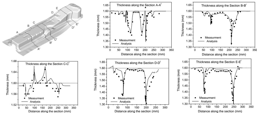
**FIGURE 13.** Comparison of the thickness distribution along the designated section for the experimental verification.
