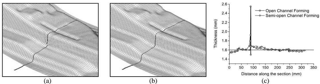
**FIGURE 7.** Comparison of the deformed shape and thickness distribution with respect to the initial blank: (a) open channel type; (b) semi-open channel type; (c) comparison of the thickness distribution
