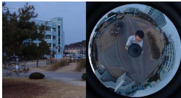
Figure 1: compared to traditional cameras (left), catadioptric systems (right) can gather much more information from the environment, such as a higher number of parallel lines that also lie in different directions.
