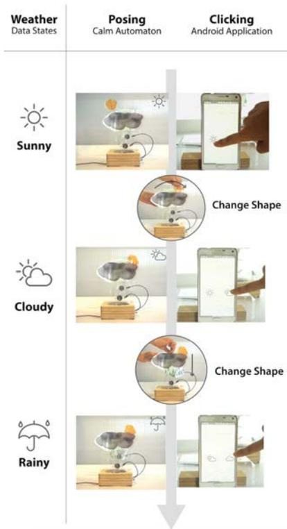
**Figure 3:** Users customize the animation by mapping states. A state is selected on a mobile phone application and programmed using a teach-in paradigm by manually moving the motion modules into position.
