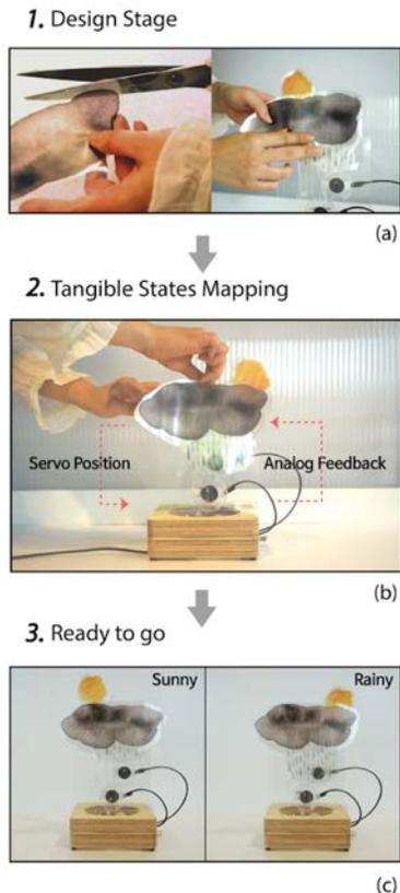
**Figure 1:** Design and mapping process with Calm Automaton (a) Cut and attach images to the motion modules, (b) Push or pull modules to map data states from the internet (c) Place at surrounding to make it move automatically
