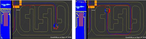
Figure 14. Localization verification with real-time AVM images: case(4) T-shape parking lot
