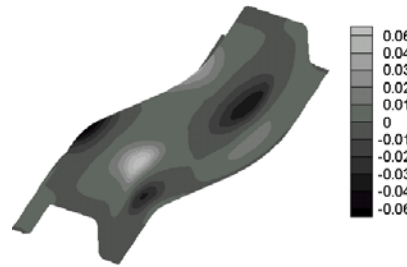
Fig. 8 Thickness strain distribution of S-Rail calculated by one step inverse analysis.
