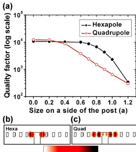
FIG. 4. (Color online) (a) Plot of the  $Q$  factors, from the contour FDTD calculation, of the hexapole and quadrupole modes with different central post side sizes. [(b) and (c)] Calculated electric field intensity profiles of the hexapole and quadrupole modes in the cross section.
