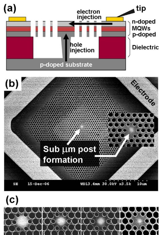
FIG. 1. (Color online) (a) Schematic diagram and (b) SEM image of the electrically driven single-cell PhC laser. At the center of the cavity, the white shadow image of the submicrometer-sized current post is shown. (c) Formation of the current post by phasing up the HCl wet-etching temperature.
