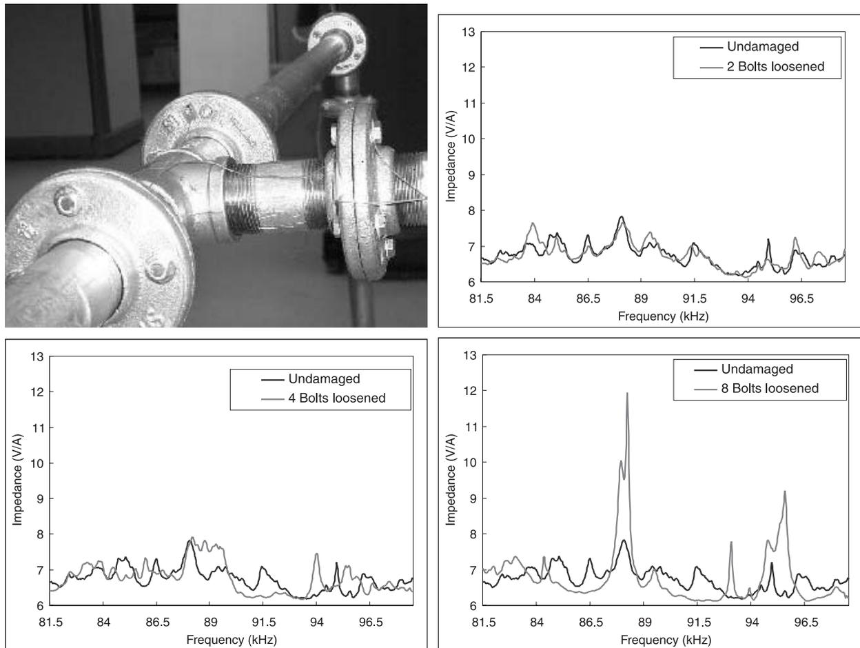
Figure 6. A pipeline experiment performed by Park et al. (2001). The impedance variation became more pronounced with increases in damage extent
