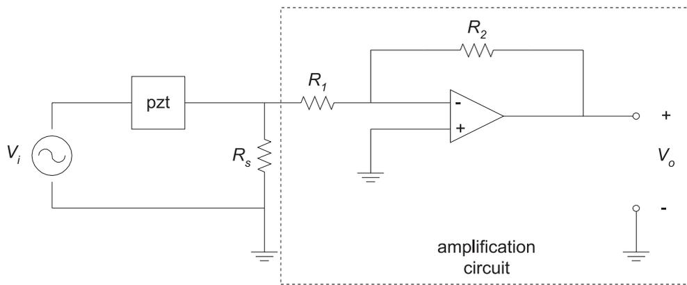
Figure 3. Impedance approximating circuit with an amplification circuit
