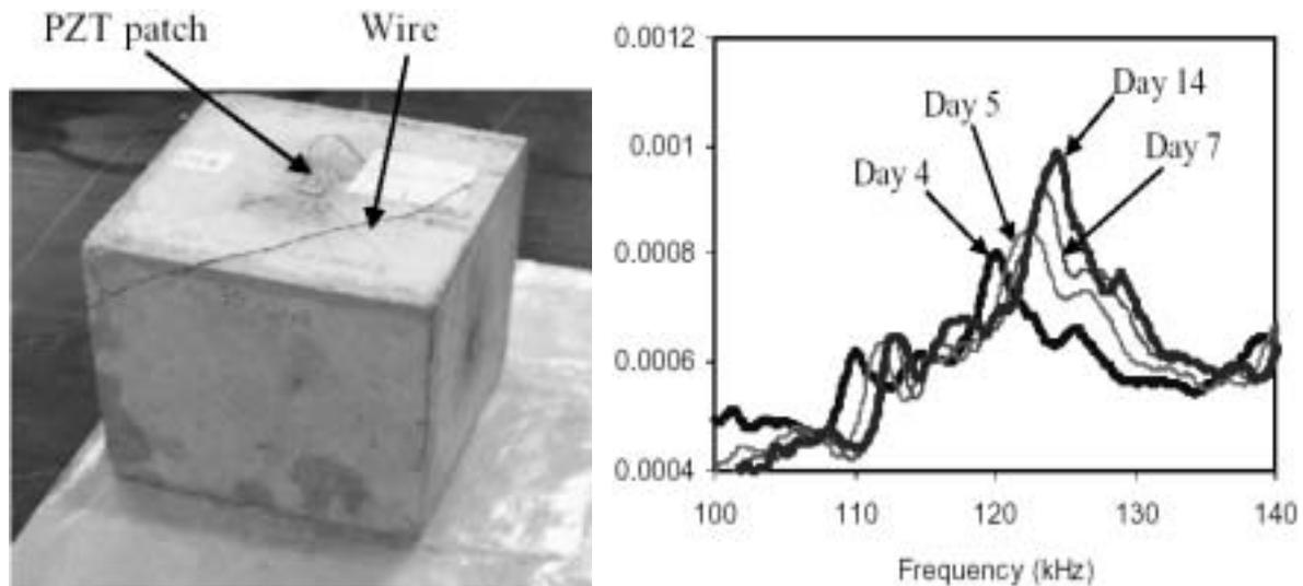
Figure 7. Bhalla et al. (2002a) show the possibility of monitoring the curing process of concrete structures. The peak shifts rightwards and becomes sharper progressively with time, which suggests the stiffness is increasing
