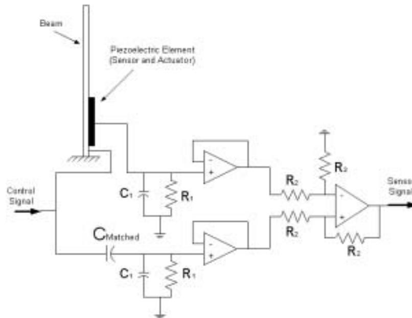
Figure 8. A schematic diagram of the self-sensing bridge circuit
