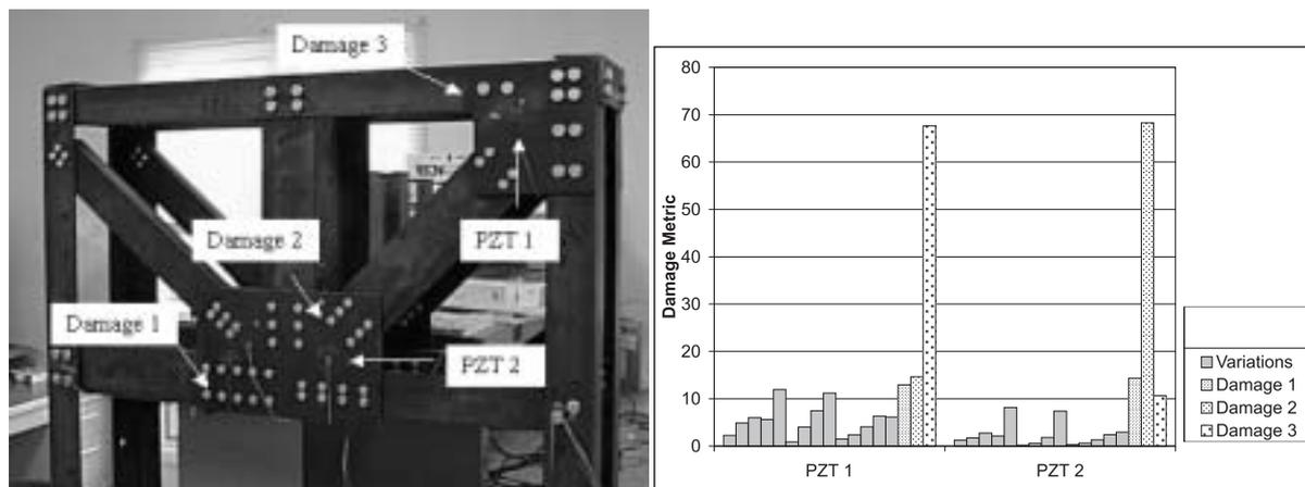
Figure 5. A quarter-scale steel bridge section (Park et al., 2000a). The damage metric shows the localized effect of the impedance method
