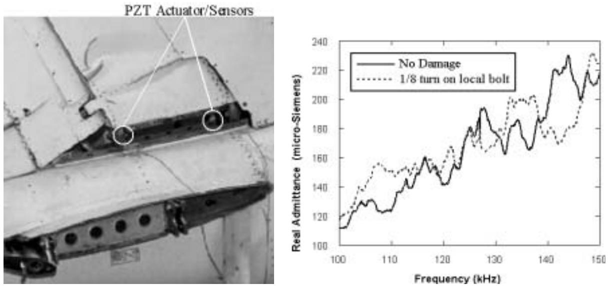
Figure 4. The integrity of the two main brackets which connect the rear fuselage to the vertical tail of a Piper Model 601P airplane were monitored (Chaudhry et al., 1995). The change in the real electrical admittance caused by loosening of the securing bolt was easily detected
