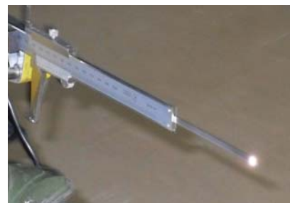
Fig. 9 The vernier calipers with reflective paper attached for parallel direction test
