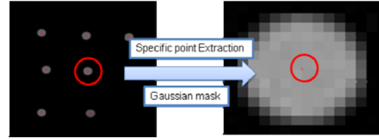
Fig. 3 Specific point (Marker reflection) extraction
