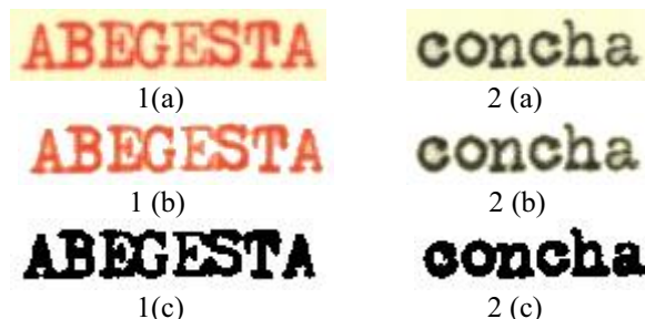
Figure 8: 1(a) and 2(a) are original colour text images; 1(b) and 2(b) are segmented foreground text in red and black ink respectively; 1(c) and 2(c) are binarized foreground text.
